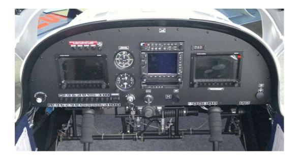
SportStar RTC is available also with the latest glass cockpit from Dynon Avionics – the SkyView System (EFIS + EMS), consisting from SkyView EFIS (Electronic Flight Information System), SkyView EMS (Engine Monitoring Display), ADAHRS (Air Data/Attitude/Heading Reference System, GPS module and Synthetic Vision System.
