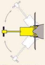
The cradle has a 5th wheel style turning that allows aircraft tug to turn full 180 degrees under aircraft wheel.
