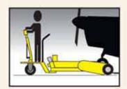
Operator can ride-on tug when staging aircraft on a ramp.
