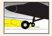
Dual nose wheel of aircraft fits securely into wheel choke on AircraftCaddy.
