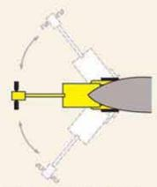
Includes 5th wheel style turning that allows AircraftCaddy to turn full 180 degrees under dual nose wheel.
